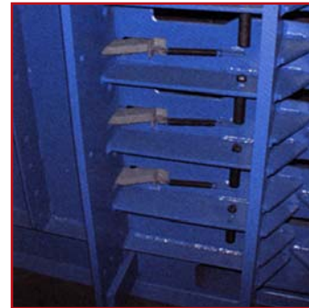
Eight spring-loaded retainer locks restrict bale spring back.
