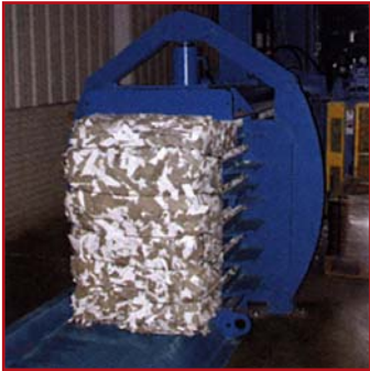
Slick material tension chamber control self-adjusts to different material.
