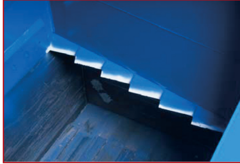
Unique tooth design reduces hydraulic shock and material jams.
