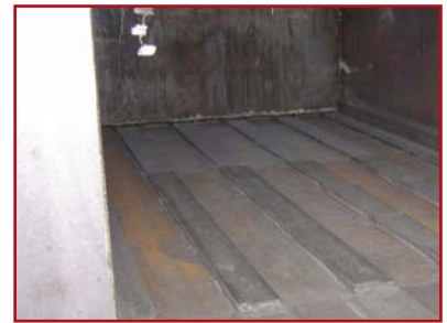
Hi-Low floor reduces material from getting under the platen.
