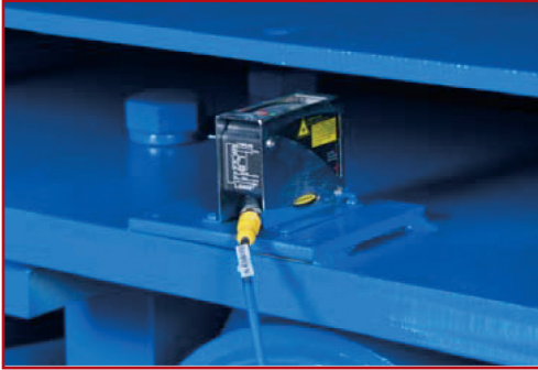
Laser linear transducer provides precise platen control – eliminating need for proximity limit switches.
