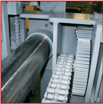
HD Double 60 chain and Gear Box. Chrome tube facilitates smooth movement of needles.
