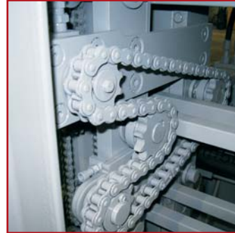
HD Single 60 chain to allow identical movement of Twister Hooks.
