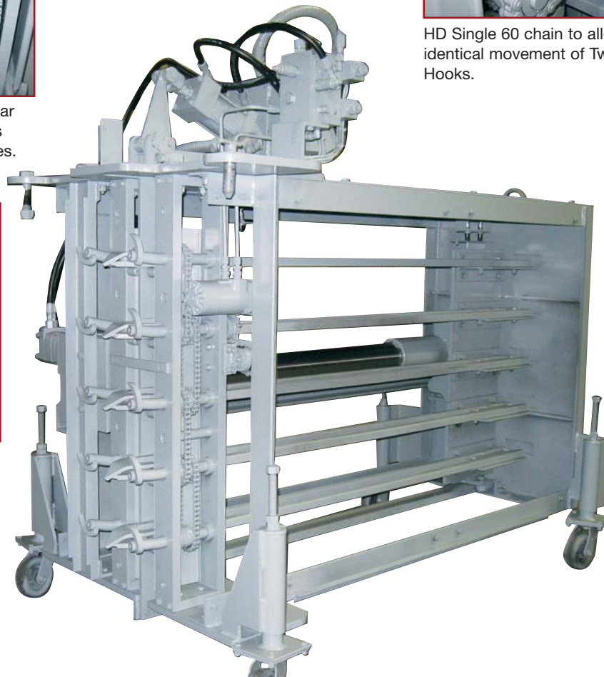
Prox. Switches for accurate positioning of needles.
