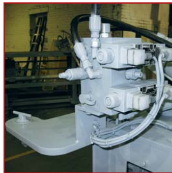
Manifold Block controls movement of Needles, Twister Hooks and Cutter Blades from a single point.
