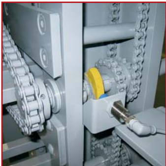
Prox. Switch for accurate position of Twister Hooks.
