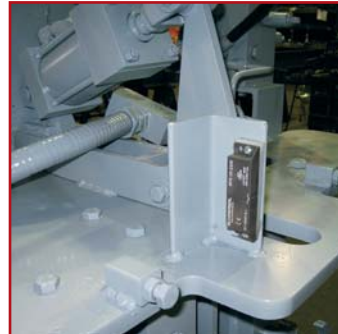
LS5 Tier in Position Safety Switch. Ensures Needles can't move when tier is not in a safe position (closed).
