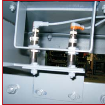
Prox. Switches for accurate positioning of needles.
