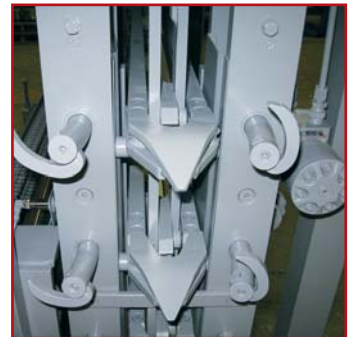
Twister Hooks and Cutter Blades located on same side as Needles.
