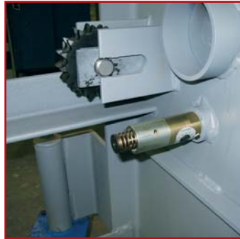
Shock absorber reduces shock on Double 60 chain.
